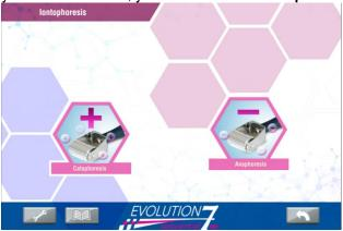
**Note:** The polarity of the DC current is pre-set, inside the unit, by a relay. Therefore, there is **no need to modify** connection of the electrodes when switching between **Cata** and **Ana**.
